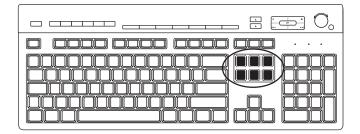
The edit keys are Insert, Home, Page Up, Delete End, and Page Down. Use these keys to insert and delete text and to quickly move the cursor on your screen. They function differently with some software programs.
